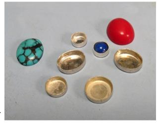
that have a sharp edge around the bottom. Burnishing the bezel over one of these stones will place a lot of stress on the stone and may cause it to crack. To avoid this, I round off the bottom edge of the stone with a diamond file (or use sandpaper on soft stones).
